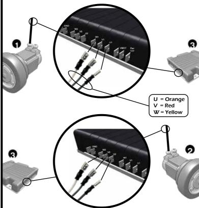
Connect drive control cable 4 to drive 8
