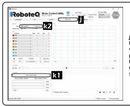
j) Click on *Diagnostics* tab k1) Select *Motor/Sensor Setup* (This will then start the autotune procedure on motor 1) k2) When completed change Channel 1 to Channel 2 and repeat step k1
